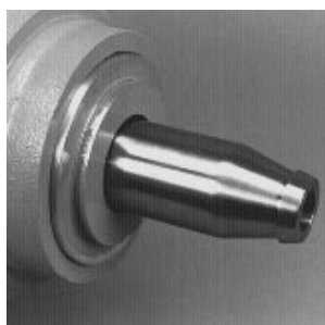
Fig. 50-12 - Install Seal Carrier (Cartridge)
