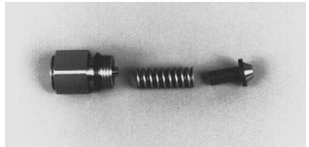
Fig. 50-21 - Charge Relief Valve Components
