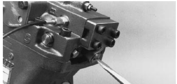
Fig. 30-6 - Adjusting Charge Pressure Relief Valve
