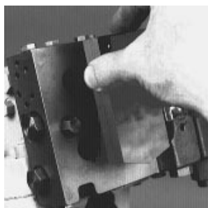
Fig. 50-37 - Remove Adapter Plate and Solenoid
