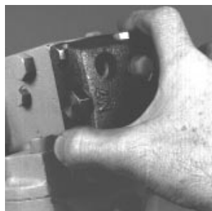
Fig. 50-47 - Install HZ Control Housing
