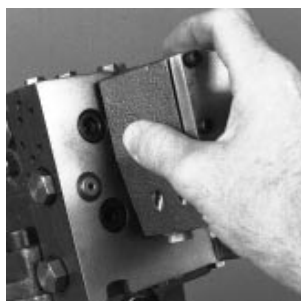
Fig. 50-59 - Remove Control Housing
