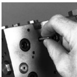
Fig. 50-61 - Remove Pilot Piston Pin
