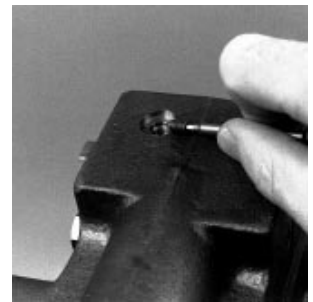
Fig. 50-146 - Servo Orifice for Maximum Displacement (T2)
