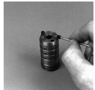
Fig. 50-148 - Servo Drain Orifices (T7 and T8)
