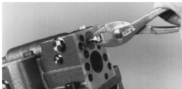
Fig. 50-26 - Remove Valve Sleeve Bore Plug
