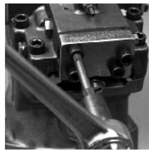
Fig. 50-22 - Remove Servo Cover Screws
