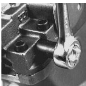
Fig. 50-14 - Remove Shuttle Valve Plugs
