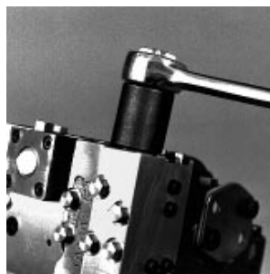
Fig. 50-128 - Remove PCOR•PC Plug
