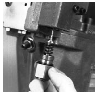
Fig. 50-127 - Remove PCOR•PC Spring and Spool Valve
