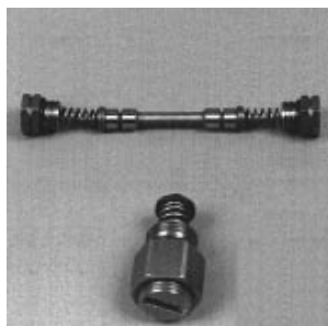
Fig. 10-2 - Loop Flushing Components
