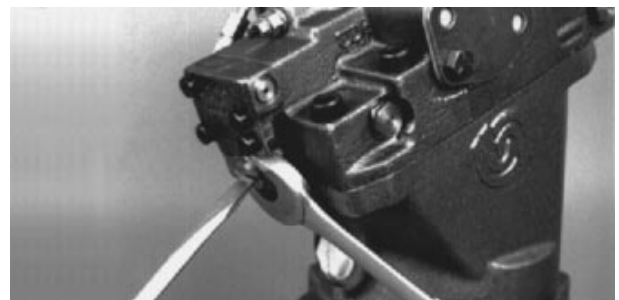
Fig. 30-7 - Tighten Charge Pressure Relief Valve Lock Nut
