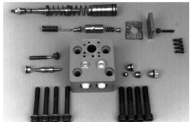
Fig. 10-30 - HC Control Components
