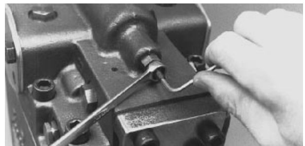
Fig. 30-18 - Adjusting Control Threshold, Types HS, HZ, H1•H2, and K1•K2
