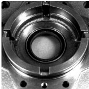
Fig. 50-5 - New Seal Installed in Flange (SAE)
