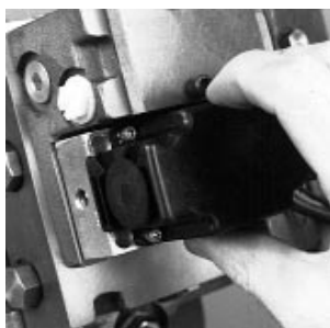
Fig. 50-109 - Install PCP onto Control
