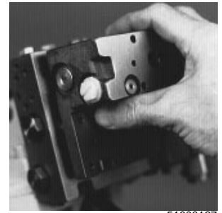
Fig. 50-102 - Install Control Housing
