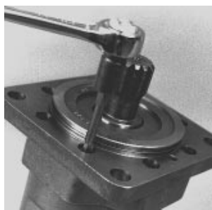
Fig. 50-2 - Remove Screws Holding Flange to Housing (SAE)
