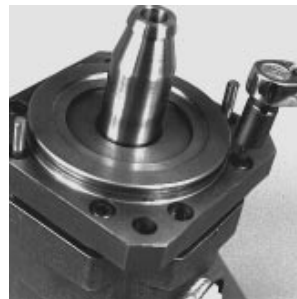
Fig. 50-6 - Install Flange onto Housing (SAE)
