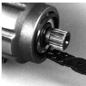
Fig. 50-13 - Install Carrier Retaining Ring (Cartridge)
