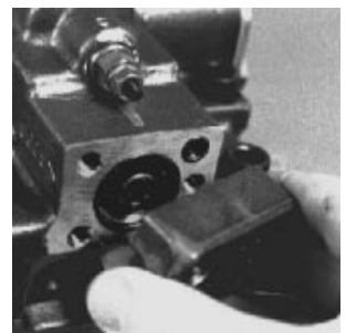
Fig. 50-23 - Install Servo Cover
