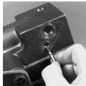
Fig. 50-147 - Servo Orifice for Minimum Displacement (T3)
