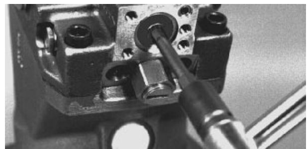
Fig. 30-11 - Torque Maximum Displacement Limiter Screw
