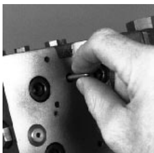
Fig. 50-99 - Remove Pilot Piston Pin
