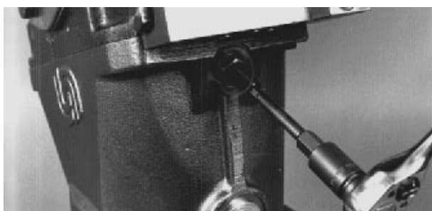
Fig. 30-9 - Rotate Minimum Displacement Adjusting Screw
