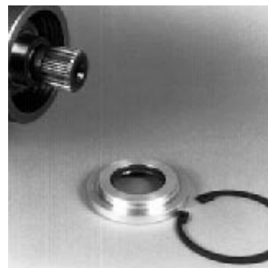
Fig. 50-10 - Seal Carrier Removed (Cartridge)
