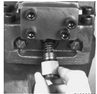
Fig. 50-20 - Remove Charge Relief Valve Plug
